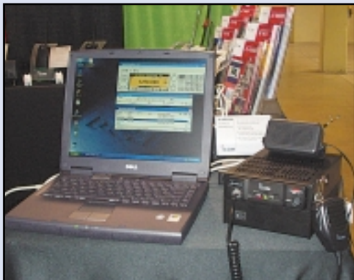
ICOM's ID-1 hooks up to a computer via a standard Ethernet connection and runs 128 kbps data as well as analog and digital voice.
