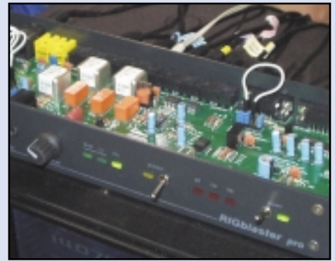
The RIGblaster Pro from West Mountain Radio is an all-in-one audio box that includes traditional RIGblaster support for sound card digital modes, plus a built-in speech processor and much more.
