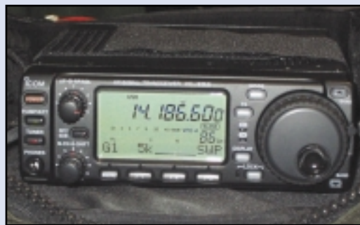
The IC-703 is ICOM's entry into the backpack radio market. The head is detachable and ICOM even offers a custom-designed backpack with special pouches, slots for cable pass-throughs, and even a rain covering.
